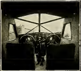
Yee windshield, improved vision, new indirectly lighted instrument panel... electric starter easily reached
